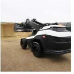
**The Loadix**, developed by ManuRob, is an innovative robotic technology for autonomous handling of agricultural materials, with a capacity of up to 30 tonnes per day.
